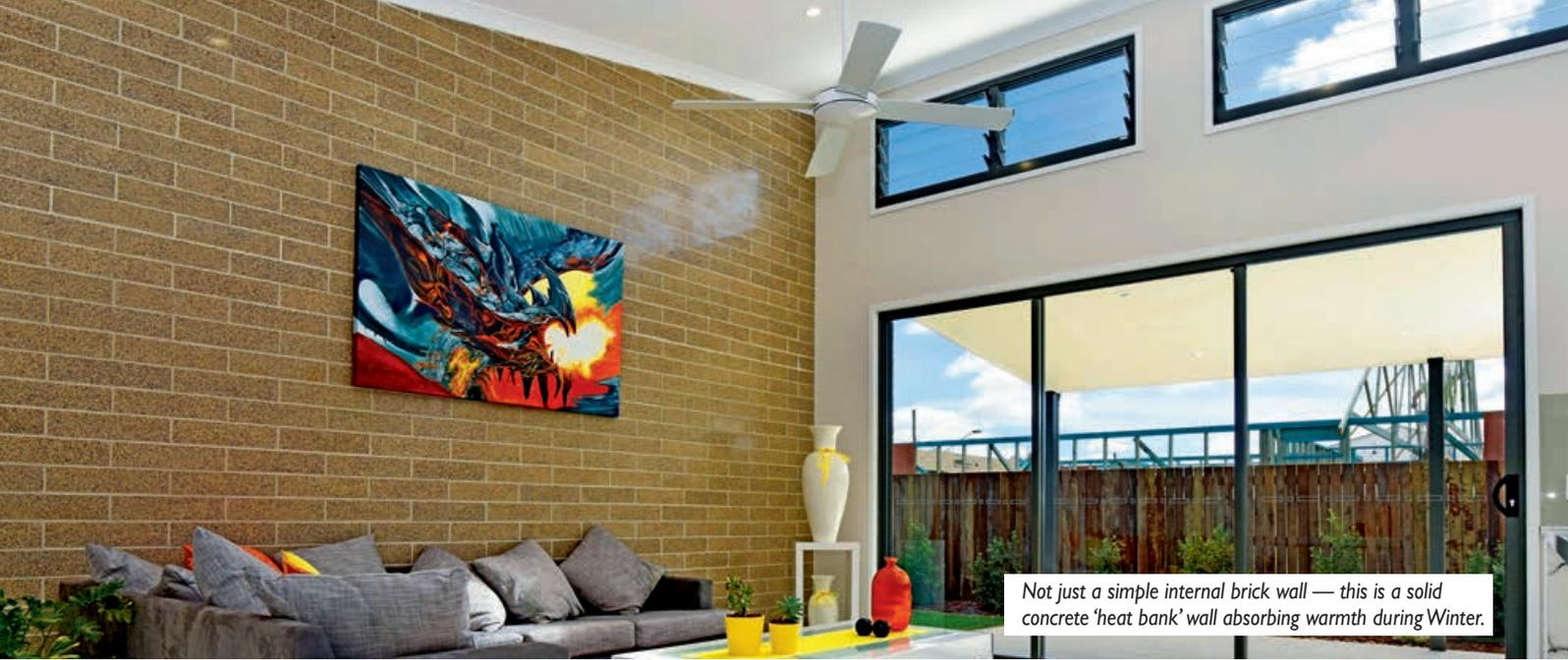
Not just a simple internal brick wall — this is a solid concrete 'heat bank' wall absorbing warmth during Winter.
